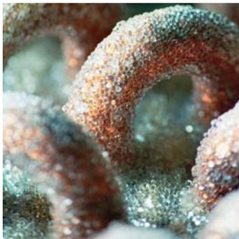
Adsorbent with silica gel coating; coating technology of the current, market-ready product series
